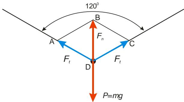
According to the third Newton's law the net force  $F_n$  is equal to the weight  $mg$ .
