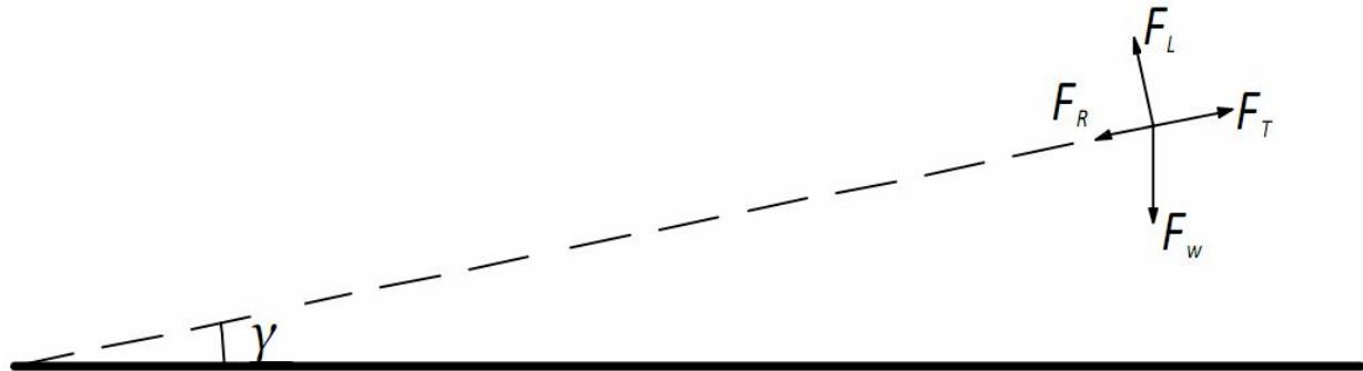
Solution: as you can see on the force diagram above, the plane is affected to such forces as weight force  $F_w = 80,000$  N, force of the air resistance  $F_R$ , wings lifting force  $F_L$ , and the moving thrust force  $F_T = 100,000$  N. All these forces are in the equilibrium, according to the third Newton's law.
