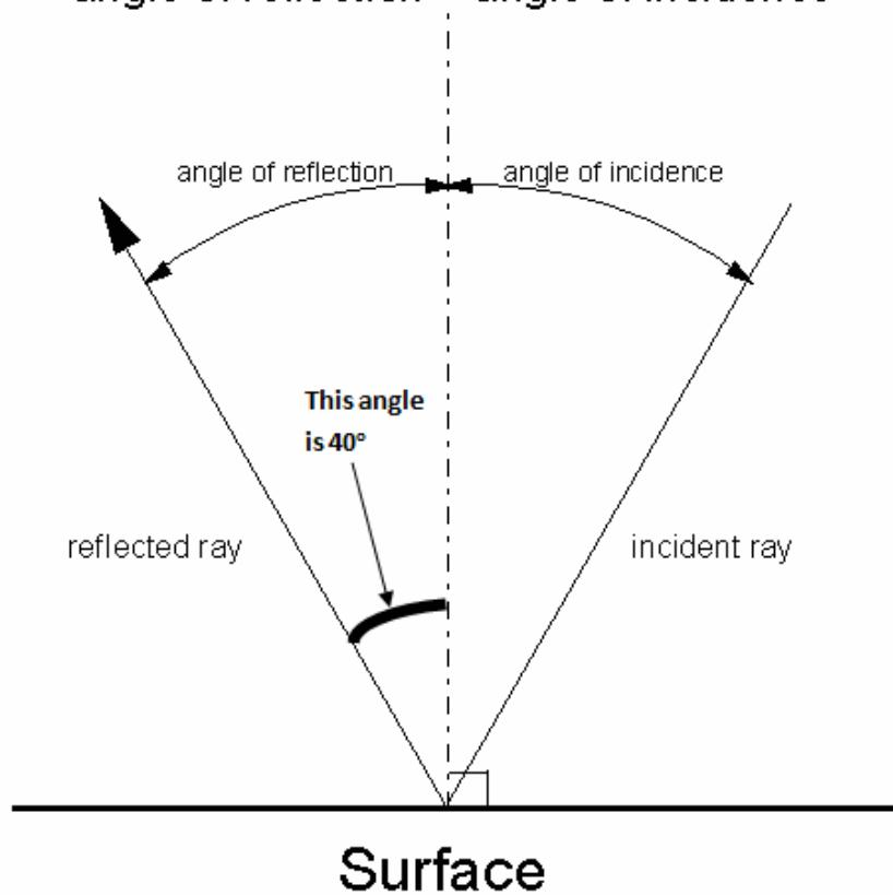
The law of reflection says that for specular reflection the angle at which the wave is incident on the surface equals the angle at which it is reflected.
