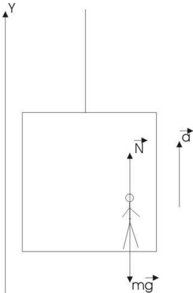
The weight of the person when an elevator at rest:
