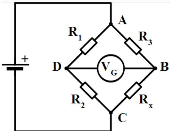
$$V_G = \left( \frac{R_x}{R_3 + R_x} - \frac{R_2}{R_1 + R_2} \right) V_s$$
