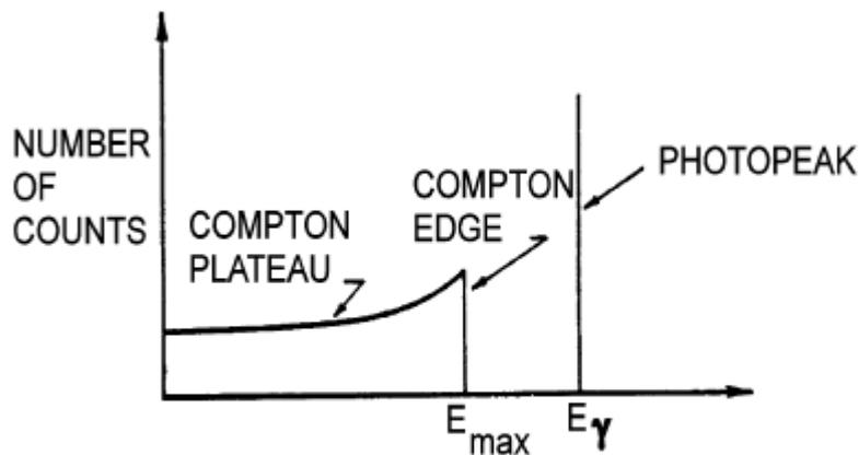
Figure 2. - Idealization of gamma-ray spectrum showing photopeak and Compton plateau
