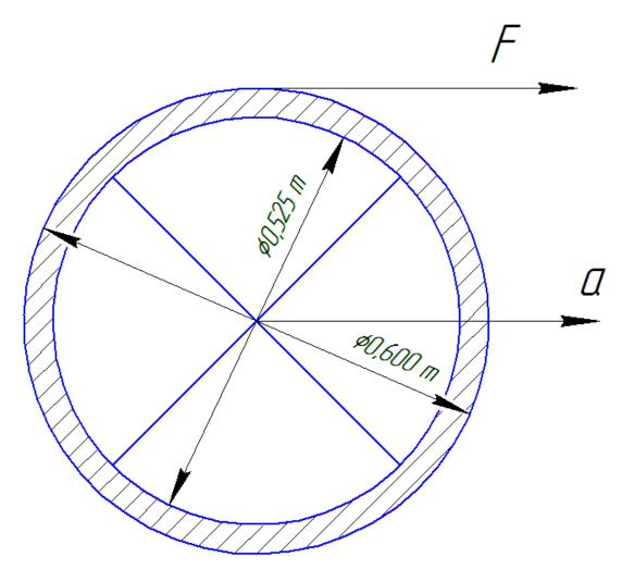
$$\tau_{net} = \frac{dL}{dt} = \frac{dI\omega}{dt} = \frac{Id\omega}{dt} = I \cdot \alpha = 7.5 Nm$$
