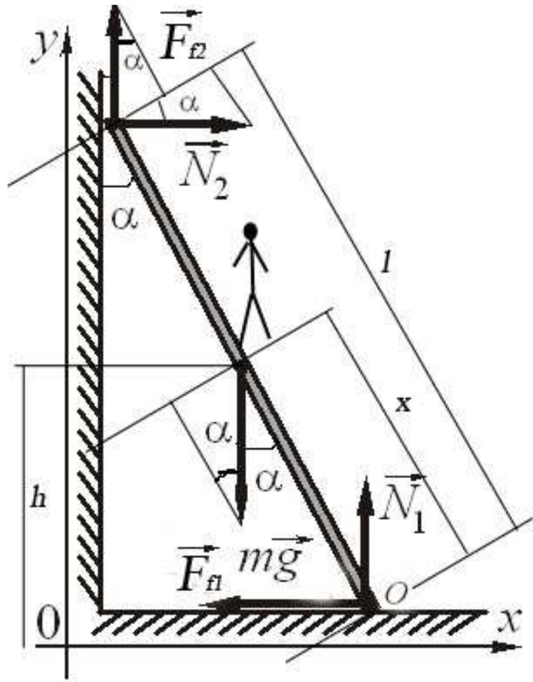
The necessary conditions for mechanical equilibrium for a system of particles.
