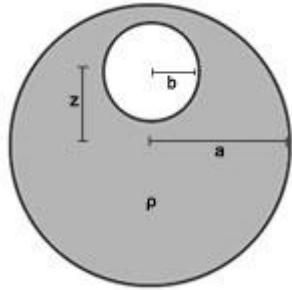
The electric field inside the cavity is going to be the superposition of the field due to the uncut sphere plus the field due to a sphere the size of the cavity with a uniform charge density of  $-\rho$ . The key to solve this problem is to calculate the electric field of each sphere in a different coordinate systems.
