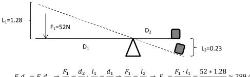
$F_1 d_1 = F_2 d_2 \rightarrow \frac{F_1}{F_2} = \frac{d_2}{d_1}; \ \frac{l_1}{l_2} = \frac{d_1}{d_2} \rightarrow \frac{F_1}{F_2} = \frac{l_2}{l_1} \rightarrow F_2 = \frac{F_1 \cdot l_1}{l_2} = \frac{52 * 1.28}{0.23} \approx 289.4 \ N_2 = \frac{1}{10} = \frac{1}{10}$
