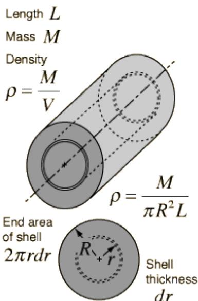
The expression for the moment of inertia of a solid cylinder can be built up from the moment of inertia of thin cylindrical shells. Using the general definition for moment of inertia:
