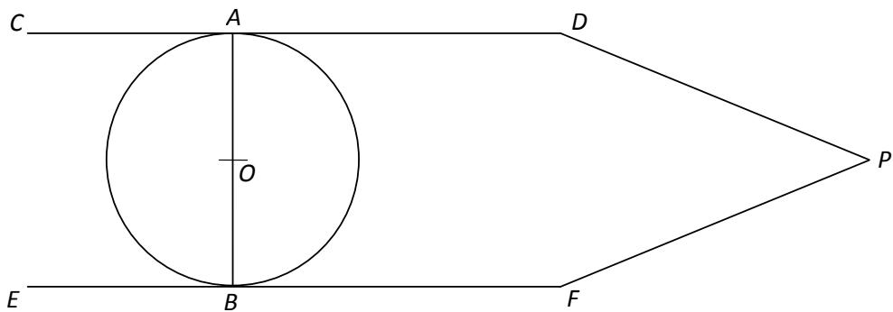
Since the tangent  $CD$  has only one common point  $A$  with the circle, then  $OA$  is the shortest distance from the center  $O$  to any point of the tangent  $CD$ , and hence the diameter  $AB$  is perpendicular to the line  $CD$  and *vice versa*. Similarly, the tangent line  $EF$  is perpendicular to the diameter  $AB$ .
