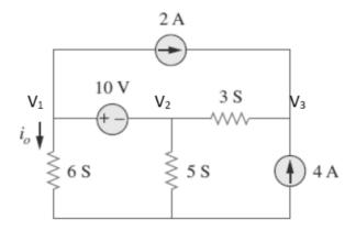
Nodes 1 and 2 form a supernode so that  $v_1 = v_2 + 10$  (1)
