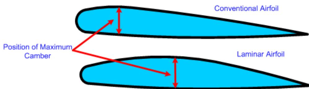
Two types of airfoils commonly used are the laminar and conventional airfoils; as a rule, the laminar foil is faster, but the cost is more adverse stalling characteristics. The two types differ with respect to location of the maximum camber—while the maximum camber on a conventional airfoil is located 25% behind the leading edge, the laminar maximum camber is located at 50% chord.
