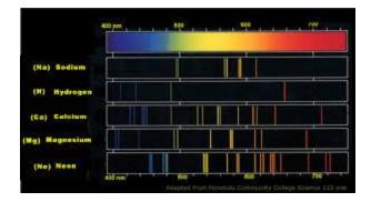
The atomic spectra of Sodium, Hydrogen, Calcium, Magnesium and Neon.
