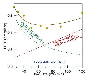
Figure 1: HETP dependence on flow rate. Points represent experimental data, full dark goldenrod line is the fit to Van Deemter equation. Green dash and firebrick dash lines represent longitudinal diffusion and mass transfer terms. Blue solid line shows Eddy diffusion level.
