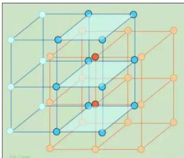
CsCl type cubic lattice is more stable under high pressure, than NaCl type cubic lattice, but less stable under high temperature. **Thus CsCl type cubic lattice can be transformed into rock salt type by applying high temperature.**
