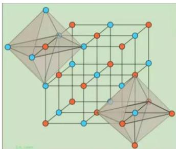
CsCl is the common model for the BCC (body-centered) structure. As with so many other structures involving two different atoms or ions, we can regard the same basic structure in different ways. Thus if we look beyond a single unit cell, we see that CsCl can be represented as two interpenetrating simple cubic lattices in which each atom occupies an octahedral hole within the cubes of the other lattice.
