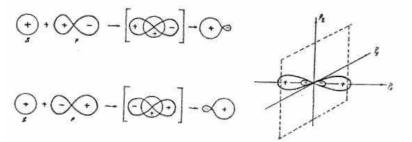
Evidently, the space orientation of these orbitals is anti-parallel that predicts linear structure of  $BeF_2$  molecule.
