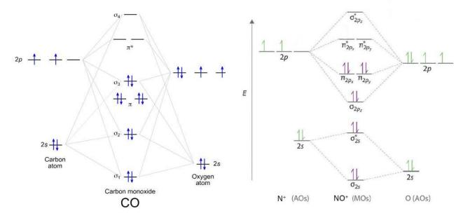
The bond order is the difference between the number of the bonding electrons and the number of antibonding electrons, divided by two. In CO and  $NO^{+}$  it is equal: (8-2)/2 = 3.
