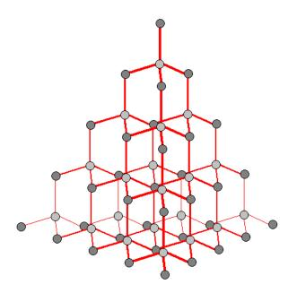
Every atom in a diamond is bonded to its neighbours by four strong covalent bonds leaving **no free electrons and no ions.** That's why diamond does not conduct electricity. The bonding also explains the hardness of diamond and its high melting point. A lot of energy would be needed to separate atoms so strongly bonded together.
