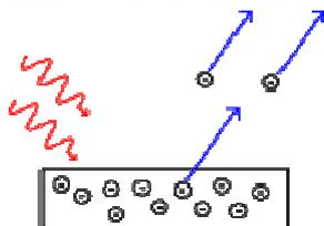
When a surface is exposed to sufficiently energetic electromagnetic energy, light will be absorbed and electrons will be emitted. The threshold frequency is different for different materials. It is visible light for alkali metals, near-ultraviolet light for other metals, and extreme-ultraviolet radiation for nonmetals. The photoelectric effect occurs with photons having energies from a few electronvolts to over 1 MeV.
