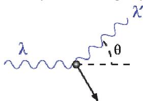
A photon of wavelength  $\lambda$  comes in from the left, collides with a target at rest, and a new photon of wavelength  $\lambda'$  emerges at an angle  $\theta$ . Energy and momentum are conserved, resulting in a reduction of both for the scattered photon.
