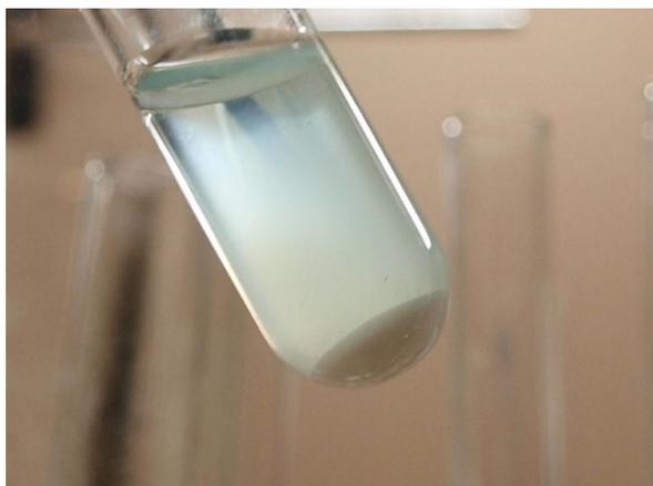
When you combine a solution of  $K_2SO_4$  with a solution of  $Pb(NO_3)_2$  a solid is formed. Chemical formula for this solid is  $PbSO_4$ .
