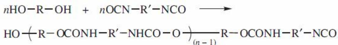
However, this is an oversimplification since other reactions are also usually involved. Foamed products such as seat cushions and bedding are the largest applications of polyurethanes. Water is often deliberately added in the production of flexible polyurethane foams. Isocyanate groups react with water to form urea linkages in the polymer chain with the evolution of carbon dioxide:
