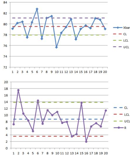
(c) The control Xbar and R charts are shown below. As we can see, Xbar chart contains points above the upper control limit line and under the lower control limit line, the R chart contains points above the UCL. Thus, the process is not in control.
